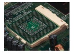
**CAUTION!** DO NOT install a heatsink on the terminator! It will cause system damage!
